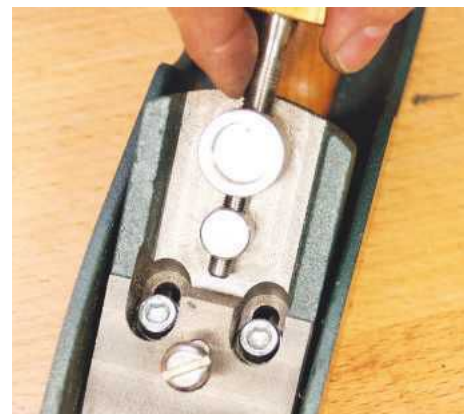
▲ The milling of the frog is very clean and finely done
